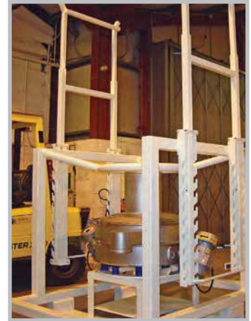
Model T1 with 'no tools' support arm adjustment and integral sifter
