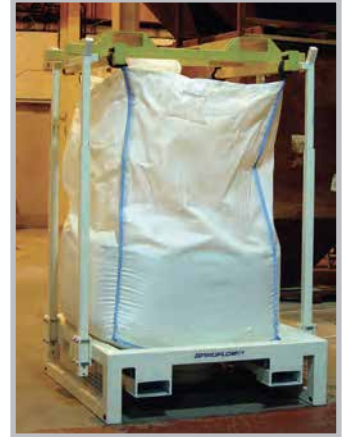
2. Loading bulk bag into top frame
