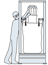
3. Liner or bag spout is attached to inflatable neck seal.
